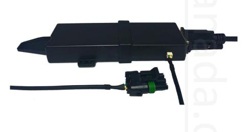
The RSA Unlock Cable is used for the unlocking of the vehicle's ECM. This cable is also required to be connected for the use of RT (Real Time) functions. This cord will be routed through the
