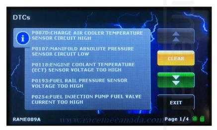
To clear the DTC's, the engine MUST be off with the ignition in the run position.
