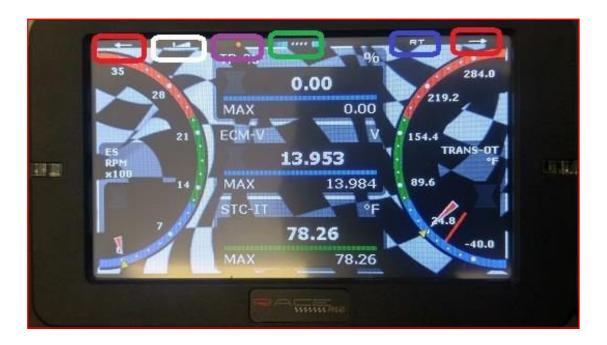
The Ultra's main gauge layout (or dashboard) come in four configurable configurations. These can be chosen from the main menu screen as ABCD, or from the gauge screen by the left and right arrows at the top of the screen.
