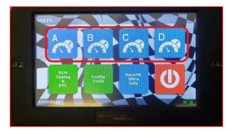
This will show a set of gauges that can be configured to show you many parameter ID's so you can monitor your trucks vitals. To change which PID is showing, touch the gauge you would like to modify.
